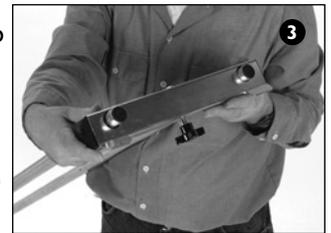
The ledge is fastened to the posts by means of a bar that runs the width of the ledge. The posts must be fitted behind this bar. That means that the bar
